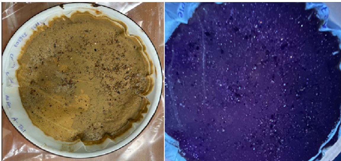
Figure 1: Left: Knelson concentrate under natural light. Right: same concentrate under UV light, showing fluorescent scheelite.
