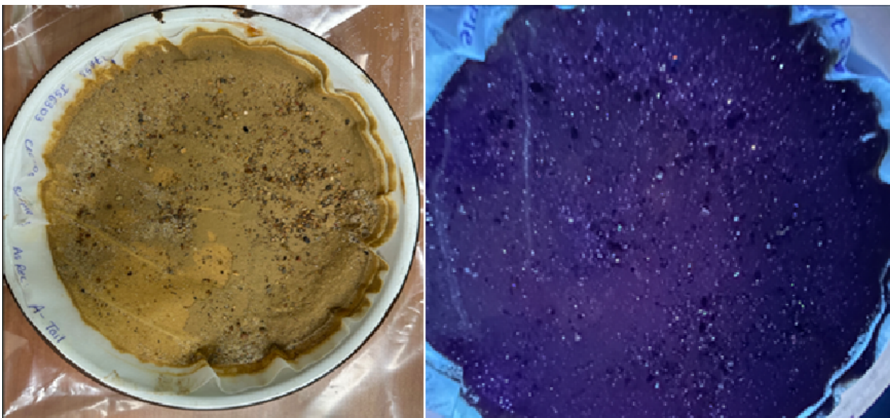
Figure 3: Left: Knelson concentrate under natural light. Right: same concentrate under UV light, showing fluorescent scheelite.
