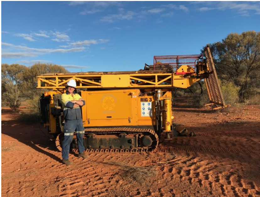
Figure 1 – MD of Metalicity Jason Livingstone with a diamond core rig positioned to drill the DCC Trend.
