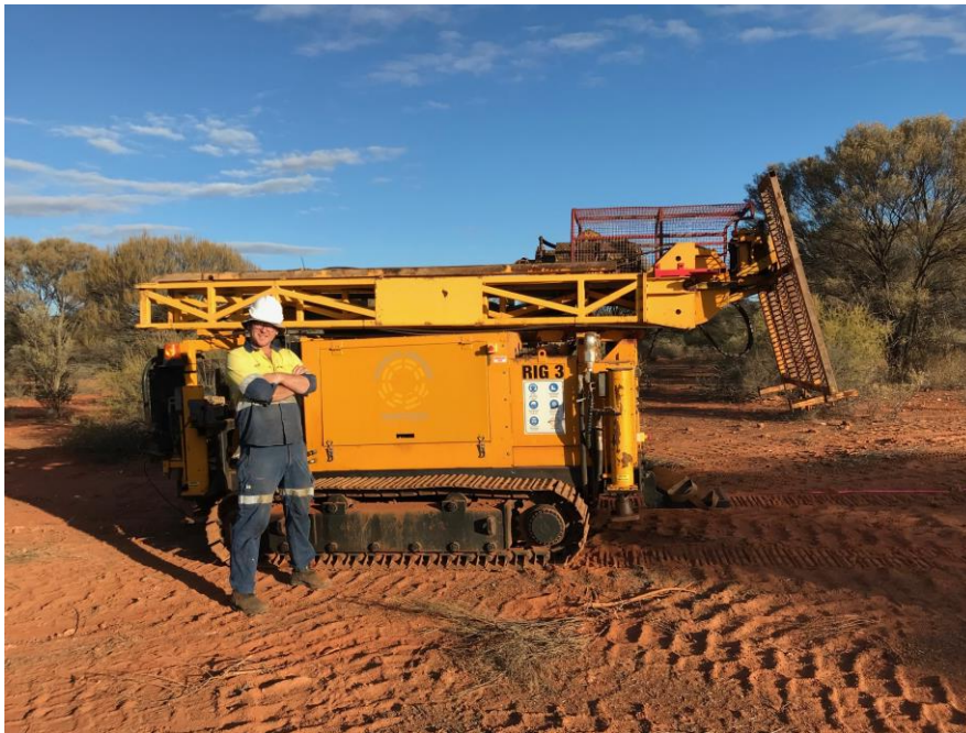
Figure 1 – A diamond core rig positioned to drill the DCC Trend.
