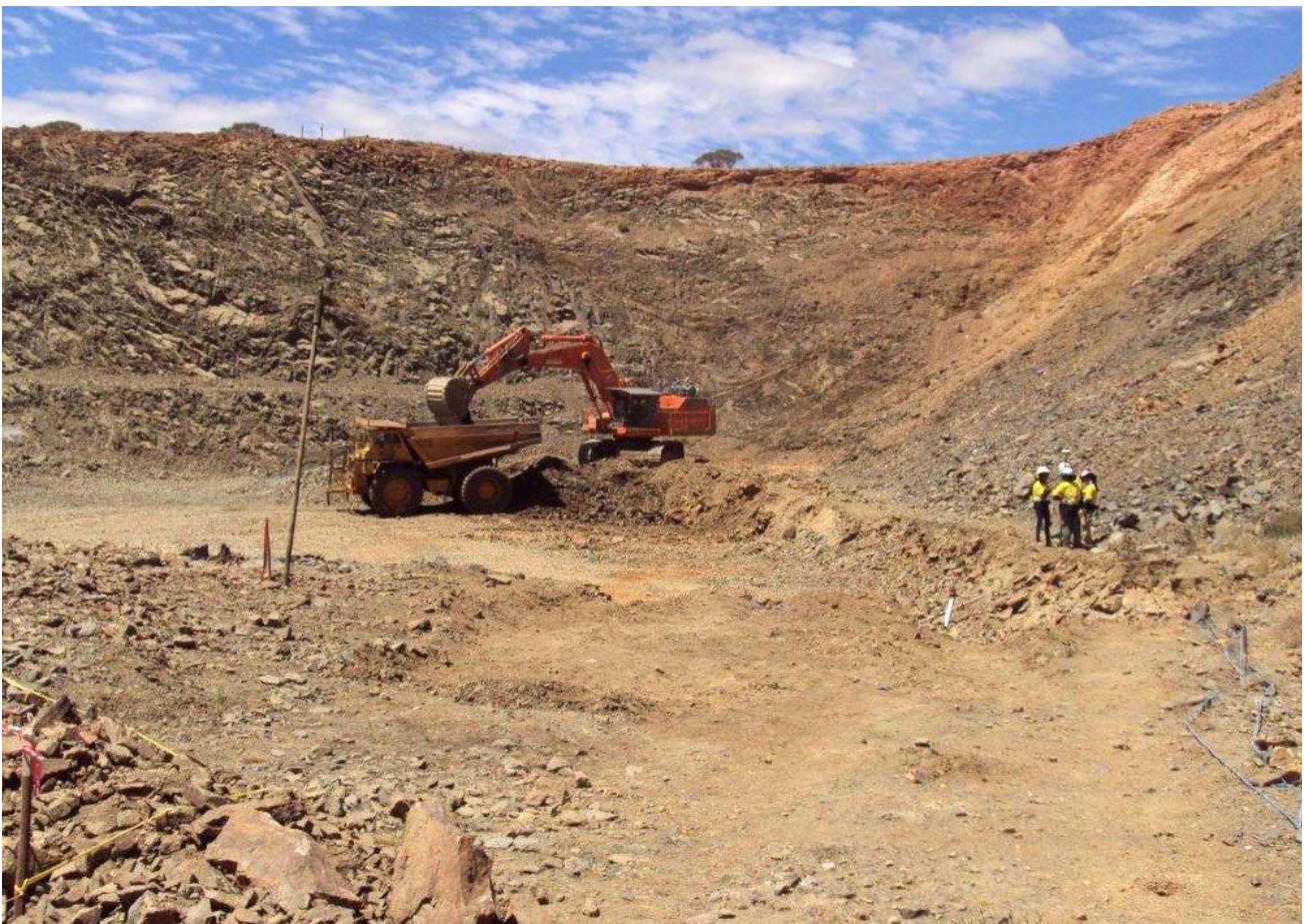
Photograph 1. Loading High Grade Ore from the Butterfly Pit. Geologists on the right being trained in spotting and controlling mining of ore to minimise mining dilution.
