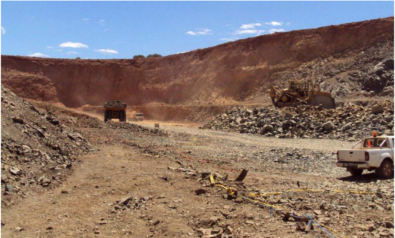
Photograph 2. Bottom of the Butterfly pit looking north-west towards the ramp. Red and green tape in the foreground delineates the ore and the yellow tape delineates the historic underground workings.
