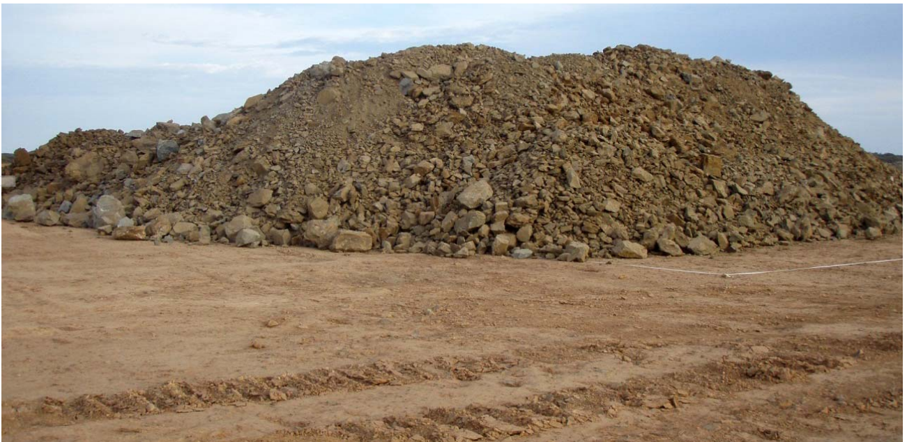
Photograph 5 High Grade ore from the Butterfly pit stockpiled ready for carting to Stone Resources Brightstar mill. Approximately 2,000t at 2.43g/t mined on the first day of ore production out of the pit.
