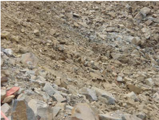
Hanging wall contact after waste has been pulled off. The angle is steeper than expected due to the heave of the blast and the next two benches the angle is expected to be a lot flatter.
