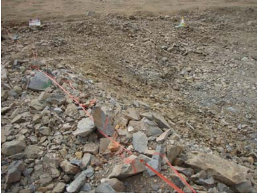
Hanging wall contact of the ore. Blue rock in picture is fly rock from stab holes in wall
