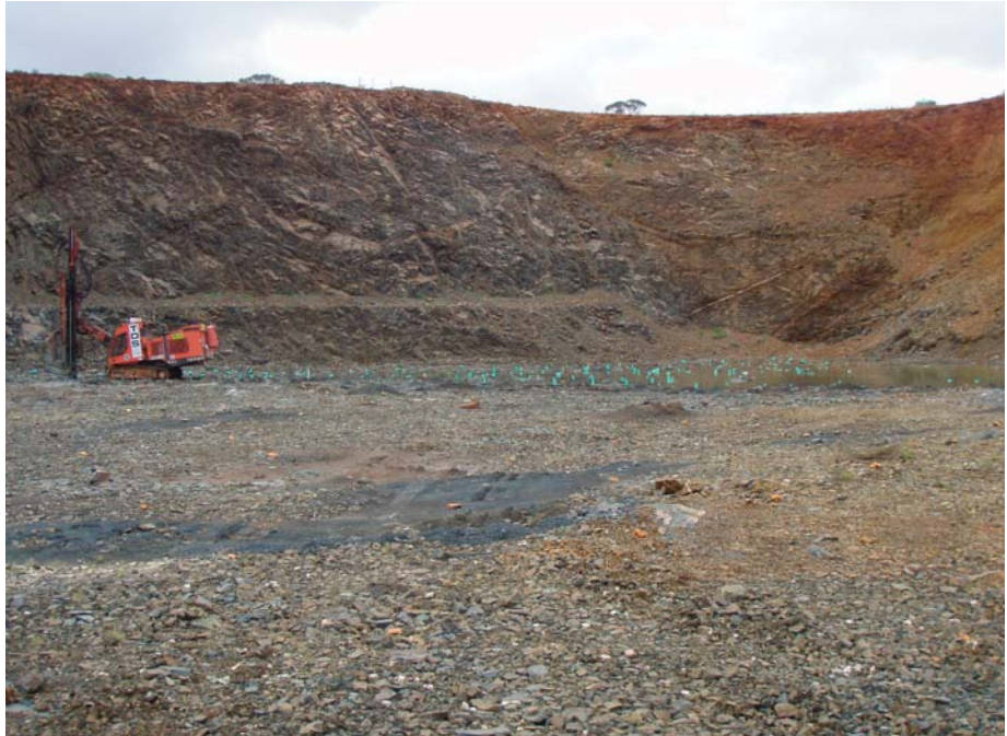
Photo 2. Blast Hole Drill Rig in the southern end of the Butterfly Pit on the first shot, water from heavy rain received over 3 days
