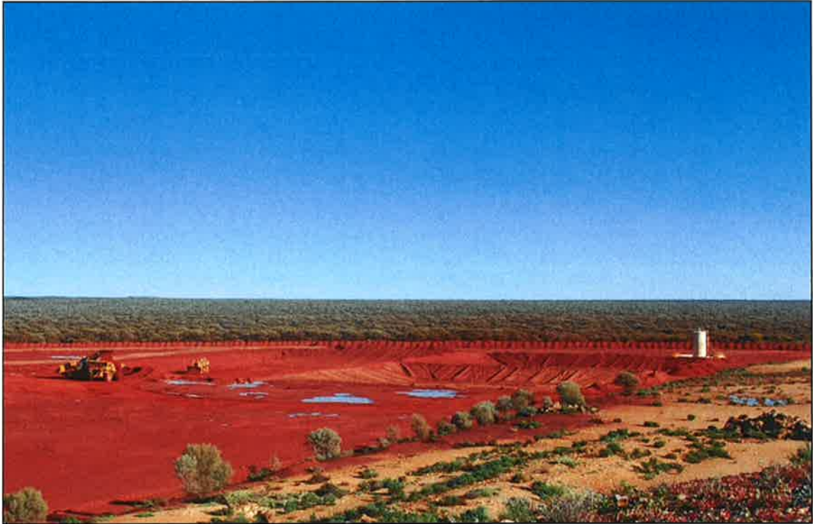
Figure 2. The Komatsu WA800-2, CAT D11N and one of the CAT 777Bs working in the stormwater pond with the pregnant and barren solution ponds and cyanide storage tank to the right.
