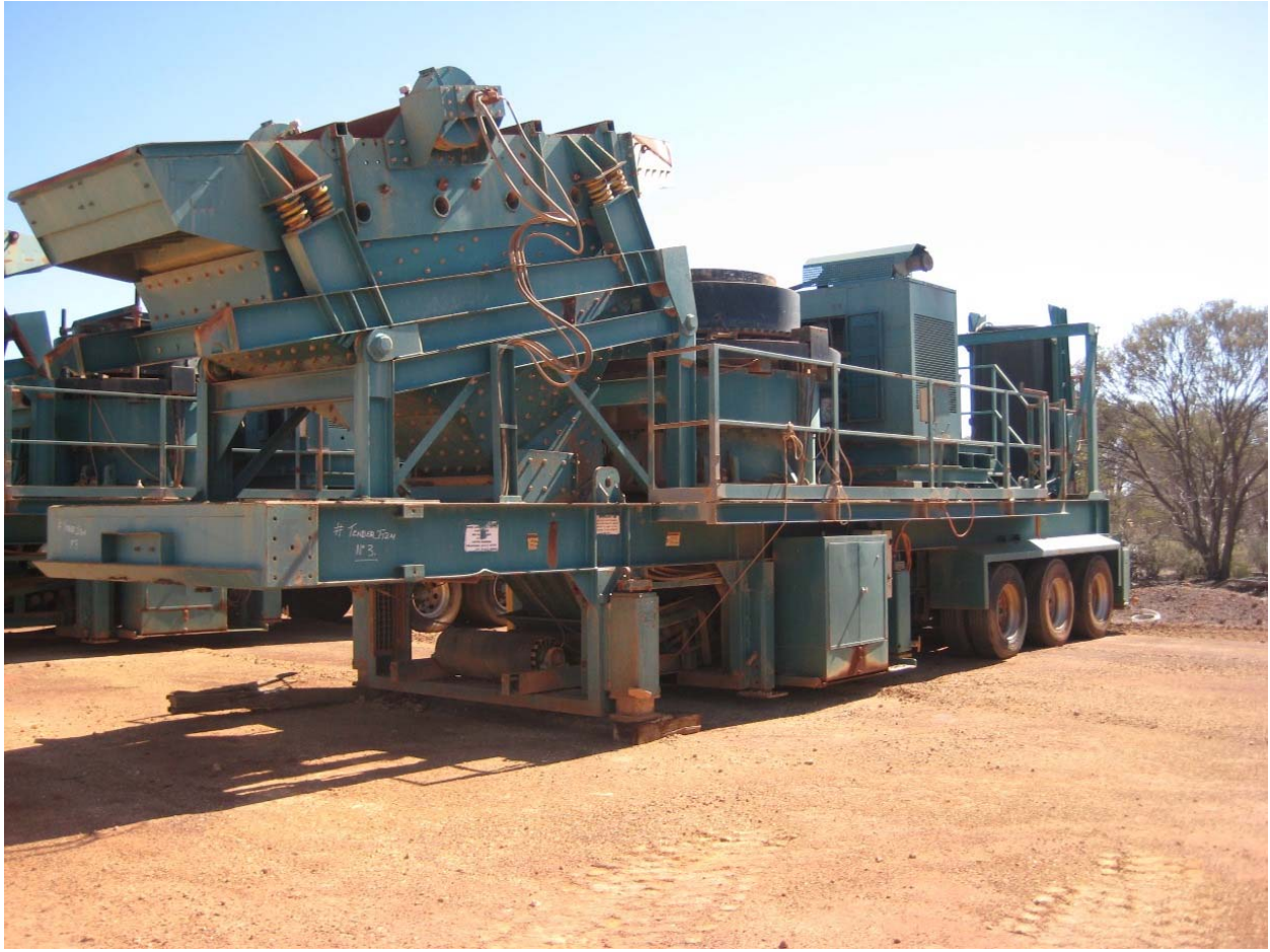
Figure 5. A component of Nex's mobile crushing/screening unit on site at Orient Well.
