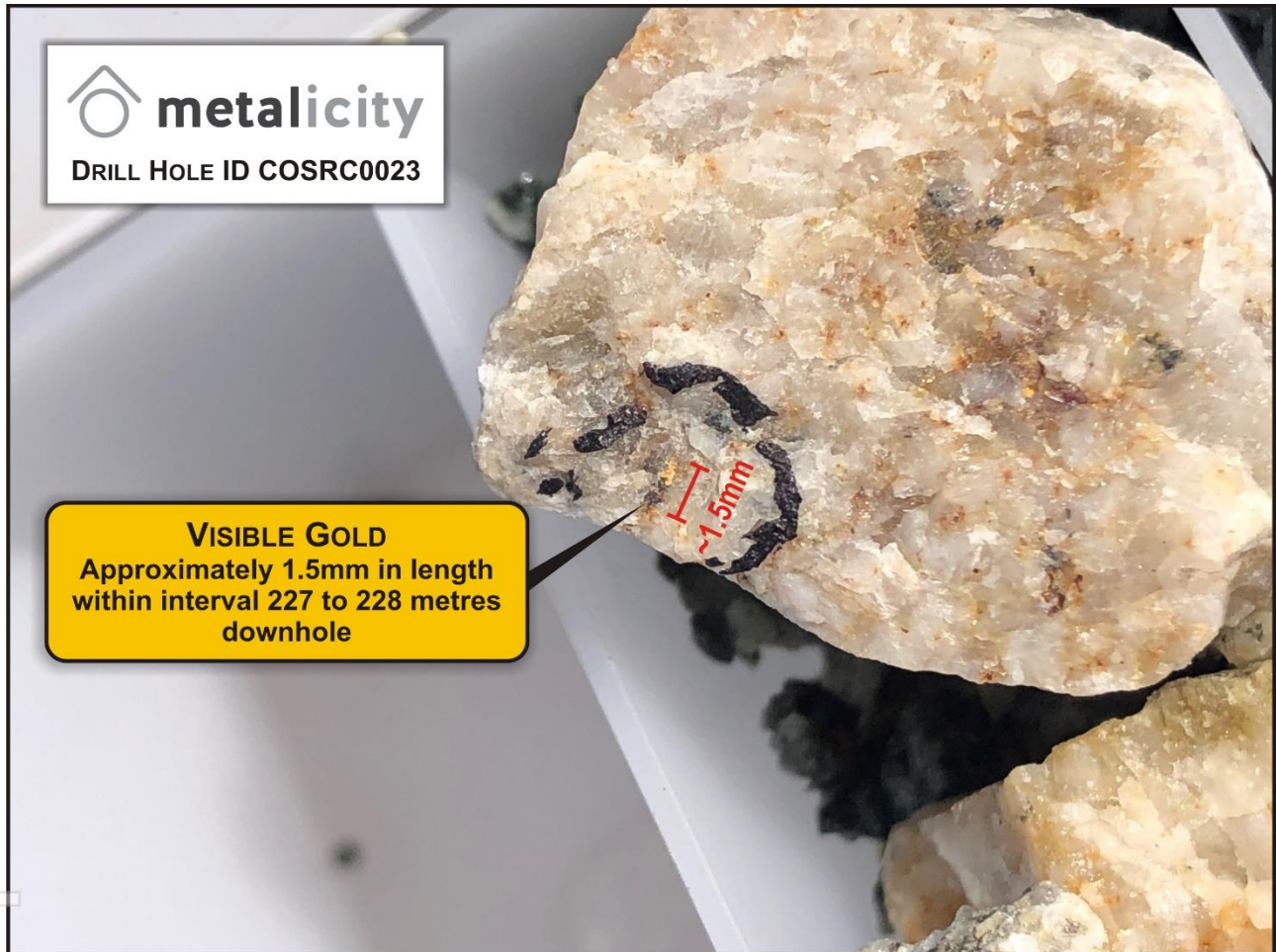
Photograph 1 – Visible gold from interval 227-228 metres in COSRC0023 at the Cosmopolitan Gold Mine.
